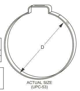
UPC 52-50 is used with aluminum core duct on the plenum take-off fitting and on the duct connector. Slide clamp over aluminum core of duct. Push duct over the take-off fitting or connector. Use tool UPC 54 to crimp clamp securely. Make sure clamp is crimped as tight as possible to insure a good connection. Tuck insulation and jacket into tape ring and secure with UL 181 aluminum tape.
